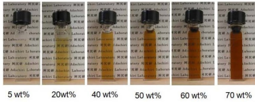
Figure 3. Dispersion of decanoic-acid-capped ceria NPs dispersed in cyclohexane
