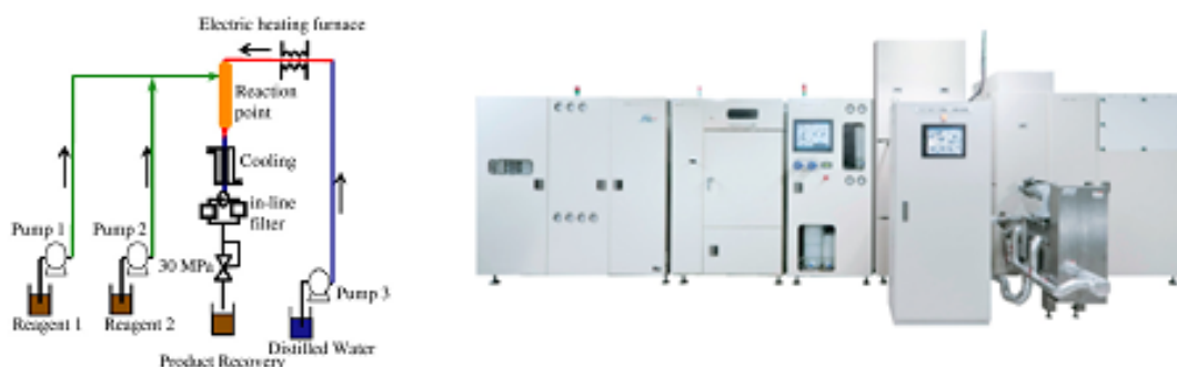
Figure 1 Flow reactor apparatus for supercritical hydrothermal synthesis (ITEC Co., LTD, Japan).
