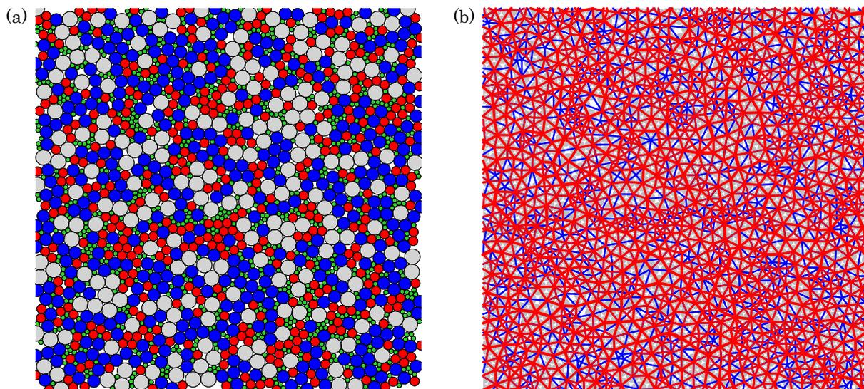
**Figure 1:** (Color online) (a) A static particle packing with an averaged overlap,  $\bar{x} = 3 \times 10^{-6} \bar{\sigma}$ , where the total number of particles is  $N = 1872$ . (b) The complete Delaunay triangulation (DT) of the static packing in (a): The red solid lines are equivalent to force-chains, where their widths are proportional to the magnitudes of contact forces. The blue solid lines connect the nearest neighbors without contacts. The gray circles represent the particles.
