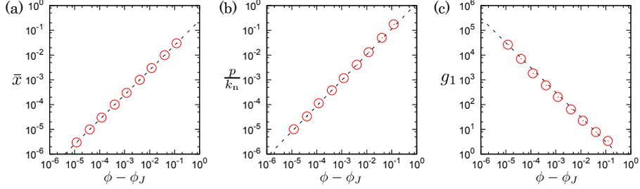
**Figure 2:** (Color online) Double logarithmic plots of the (a) averaged overlap,  $\bar{x}$ , (b) static pressure scaled by the normal stiffness,  $p/k_n$ , and (c) first peak of radial distribution function for scaled distance,  $g_1$ , where the dotted lines are power law fittings, (a)  $\bar{x} = 0.25\bar{\sigma}(\phi - \phi_J)$ , (b)  $p/k_n = 1.25 \times (\phi - \phi_J)^{1.04}$ , and (c)  $g_1 = 0.31(\phi - \phi_J)^{-1}$ , respectively.
