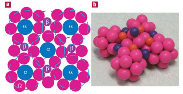
**Figure 3.** Illustrations of portions of a single cluster unit cell for the dense cluster packing model.[24]
