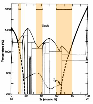
**Figure 1.** Binary phase diagram of Ni-Zr system. The shadow regions correspond to the composition ranges for the formation of metallic glasses by rapid cooling.[6]
