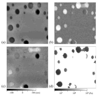
**Figure 6** The result of a force volume measurement on the same sample. (a) The force volume (apparent) height image, (b) the sample deformation image, (c) the reconstructed real height image and (d) the Young's modulus distribution image.  $^{5)}$
