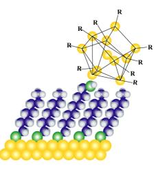
Figure 4. An atomically precise assembly of a single Au<sub>11</sub> cluster attached through a single alkanedithiolate tether molecule to a substrate with a precisely defined chemical environment has surprisingly unstable electronic structure at 4 K and 10<sup>-14</sup> torr.<sup>27</sup> We will learn how to stabilize and to predict the properties of these as well as precise assemblies with much greater complexity.
