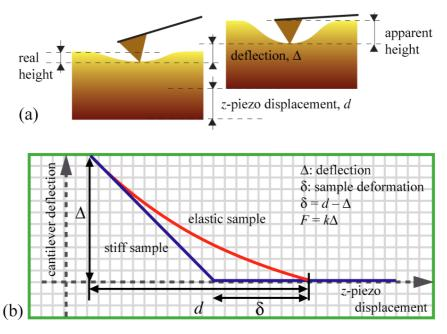
**Figure 4** (a) The schematic drawing of sample deformation for an elastic sample. (b) The comparison between force-distance curves for stiff and elastic samples.
