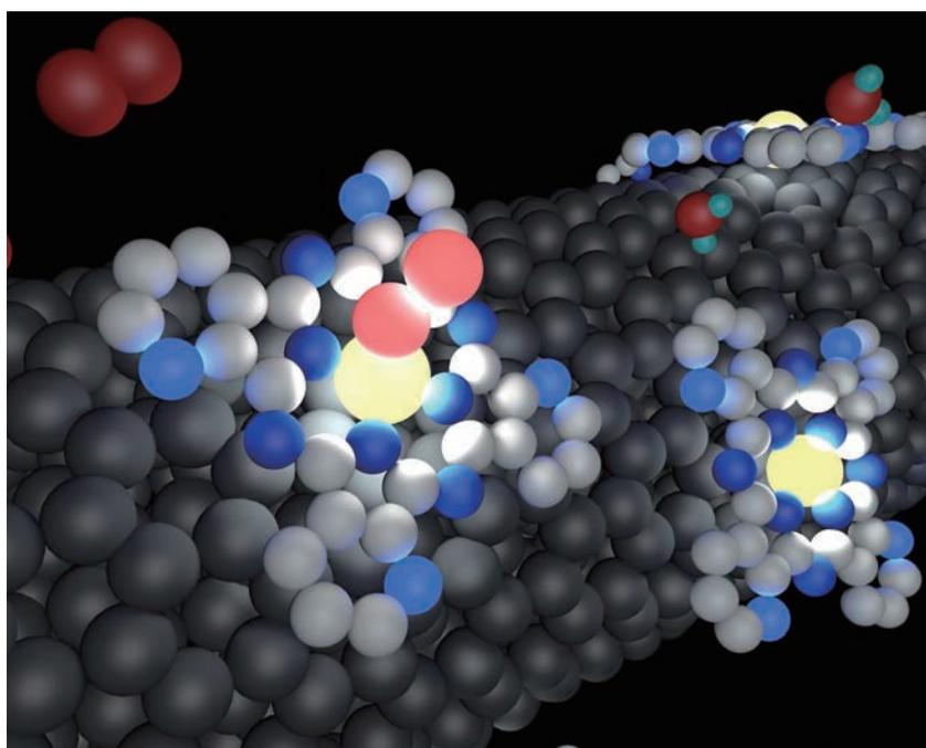
A schematic drawing showing the atomic structure of a new catalyst whose catalytic activity is higher than that of platinum-containing catalysts (gray spheres: carbon atoms in carbon nanotubes; yellow spheres: iron atoms; blue spheres: nitrogen atoms; white atoms: carbon atoms in azaphthalocyanine rings; red spheres: oxygen atoms; green spheres: hydrogen atoms).
