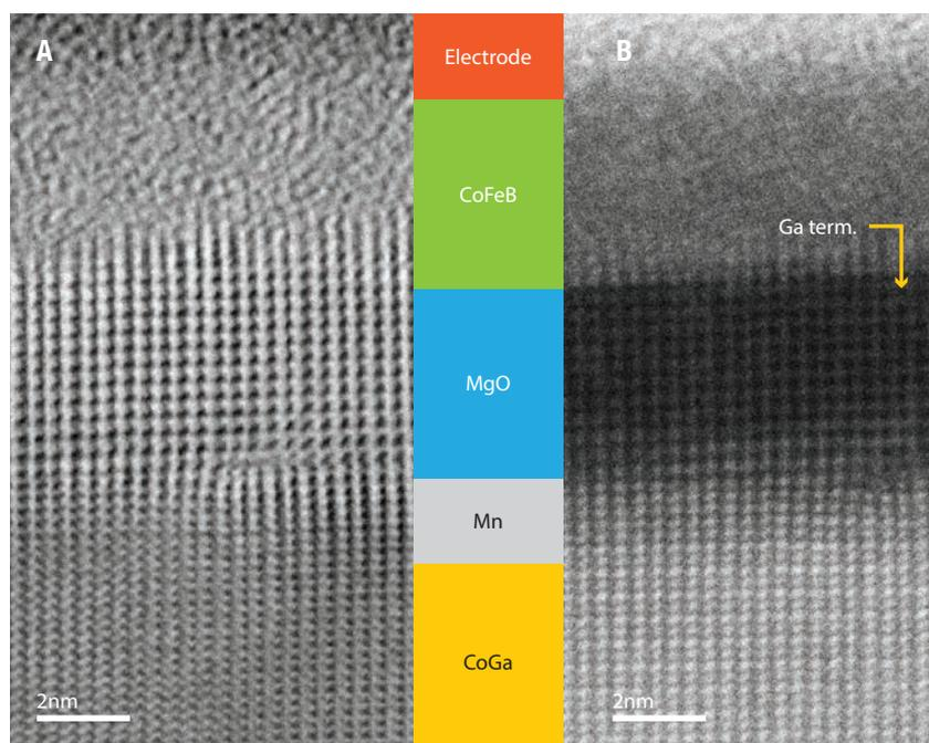
A transmission electron microscopy image (A) and a high-angle annular dark-field scanning transmission electron microscopy image (B) of the cross-section of the junction.
