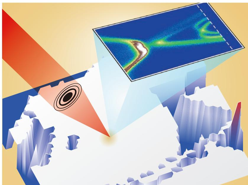
By using angle-resolved photoemission spectroscopy (ARPES) with a nanoscale beam (red ‘pencil’ on left), researchers at AIMR were able to image the domains on a multilayer topological heterostructure and determine their electronic states (blue ARPES intensity plot).
