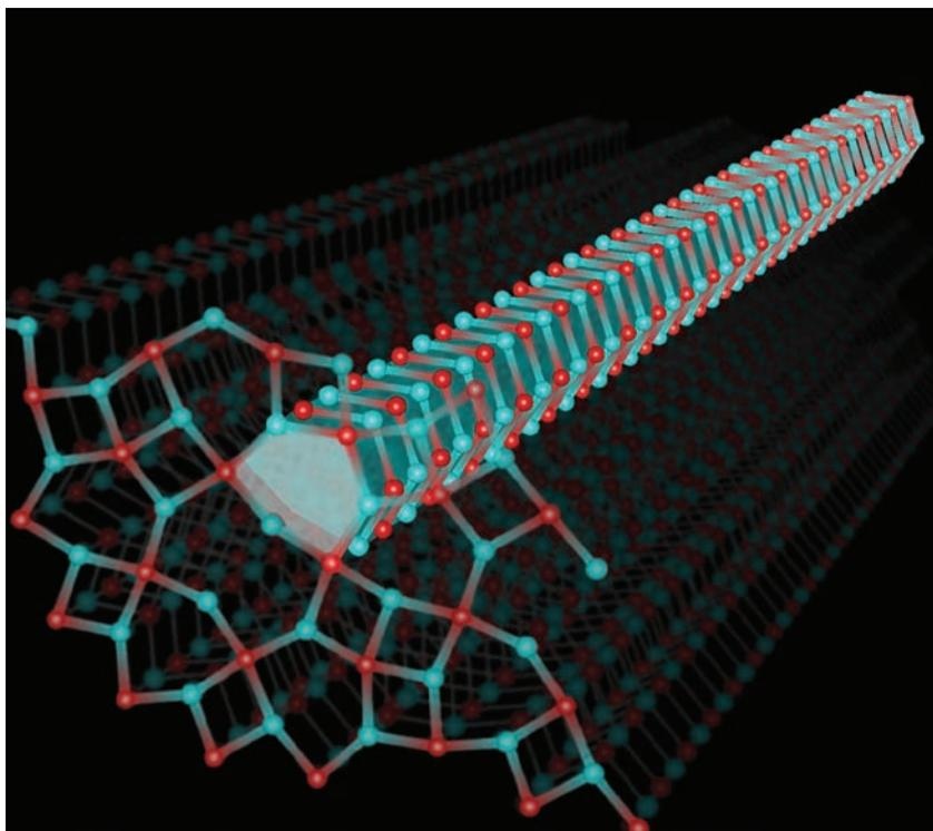
The new crystallographic phase has a random arrangement in one plane, but translation symmetry along the direction perpendicular to the plane.
