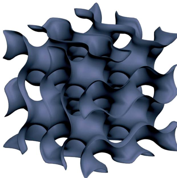
This nanoporous, graphene-based structure has both high tensile strength and ductility.
