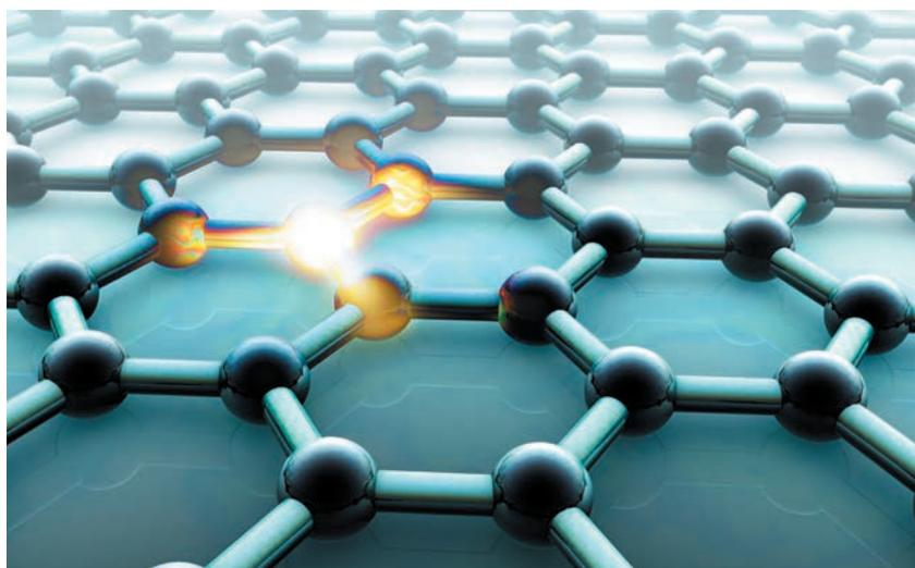
Introducing defects and chemical dopants can boost the electrocatalytic activity of graphene for the hydrogen evolution reaction.
