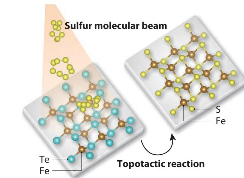
Takafumi Sato and his team produced a monolayer of iron sulphide for the first time by using molecular-beam epitaxy to deposit sulfur atoms on a monolayer of iron telluride (left image) and then inducing a topotactic reaction to replace the tellurium atoms in the monolayer with sulfur atoms.
