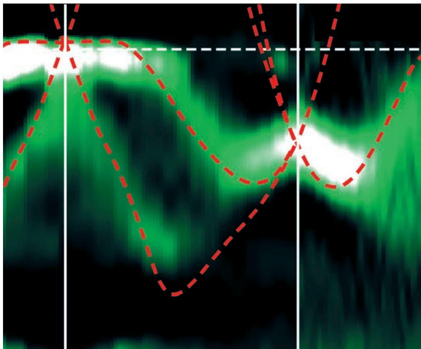
An angle-resolved photoemission spectrum that reveals the existence of one of the two new kinds of fermions discovered in cobalt silicide.
