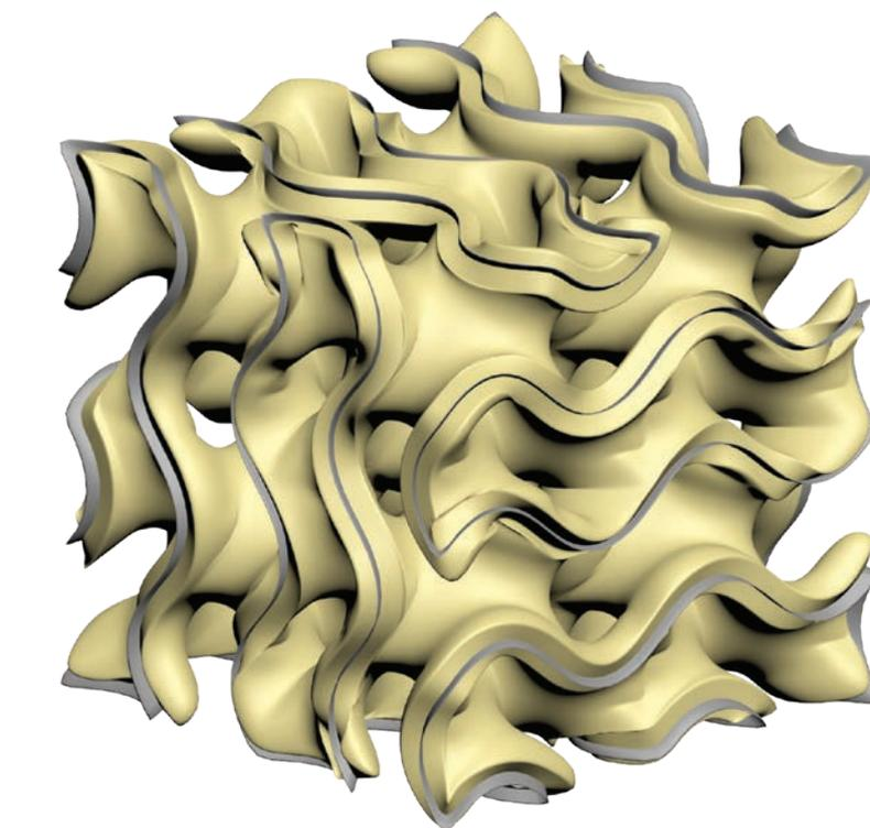
Nanoporous nitrogen-doped graphene contains a very large surface area that helps it to store lithium.
