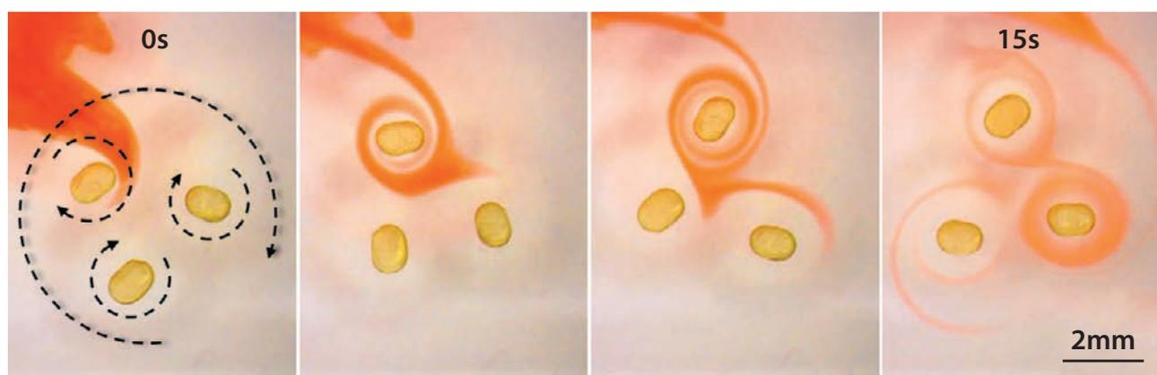
Three liquid droplets that have a permanent magnetization can be made to rotate in unison by applying a rotating magnetic field. The orange dye shows the swirling fluid flow created by the rotating droplets.
