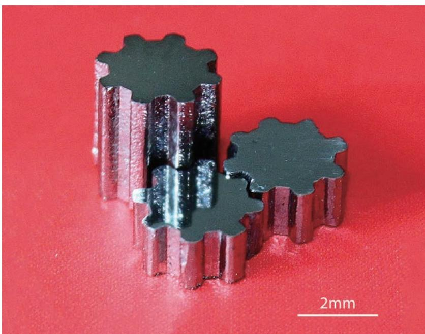
The mechanical properties of metallic glasses make them suitable for small components such as microgears.
