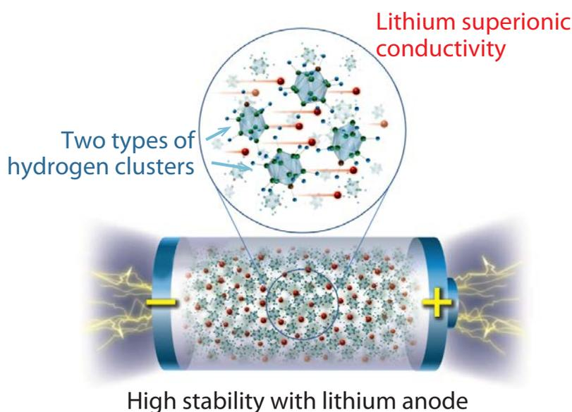
A complex hydride that has two types of hydrogen clusters exhibits both a high lithium ion conductivity and an excellent stability with lithium metal anodes.
