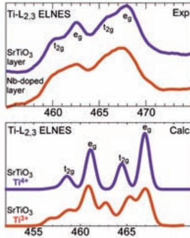
Fig. 12. (top) Experimental and (bottom) theoretically calculated Ti-L<sub>2,3</sub> ELNES obtained from the SrTiO<sub>3</sub> layer and the Nb-doped SrTiO<sub>3</sub> layer in the SrTiO<sub>3</sub>/Nb-doped SrTiO<sub>3</sub> superlattice. The calculations were made by the first principles relativistic multielectron method.
