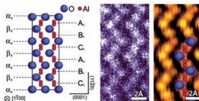
Fig. 9. (a) Atomic structure model of sapphire projected along  $[1\bar{1}00]$  direction, (b) HAADF- and (c) BF-STEM images of a sapphire single crystal viewed from  $[1\bar{1}00]$  direction [16].
