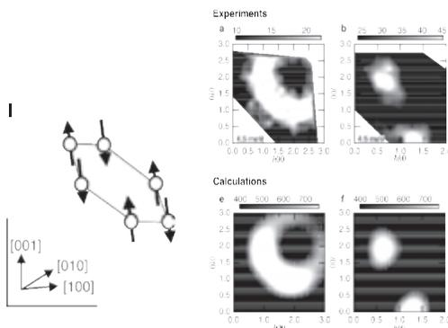
Fig. 5. The upper two panels show contour images of single-crystal inelastic neutron scattering intensities of  $\text{MgCr}_2\text{O}_4$  measured at 4.5 meV at 6 K in the  $hk0$  zone(left) and the  $hhl$  zone(right), respectively. The lower two panels show the corresponding calculated images based on the spin correlation confined in the hexamer shown in the left.
