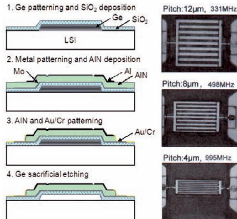
Fig. 1.1. Multi-band Lamb wave resonator for time-frequency generation.
