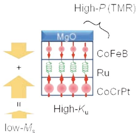
Fig. 7. Concept of perpendicular synthetic ferromagnetic structure
