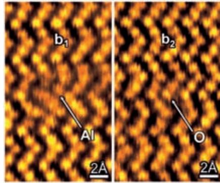
Fig.10. BF-STEM images of the core structures of the dissociated basal dislocations ( $b_1$  and  $b_2$ ), indicating that each core terminates at Al and O, respectively [16].
