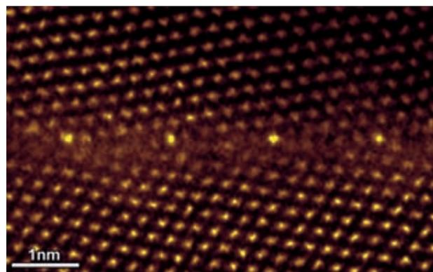
Fig. 7. HAADF-STEM image of Y-doped  $\Sigma$  31 [0001] tilt grain boundary in alumina. The brightest columns indicate the presence of the heavy Y ions.
