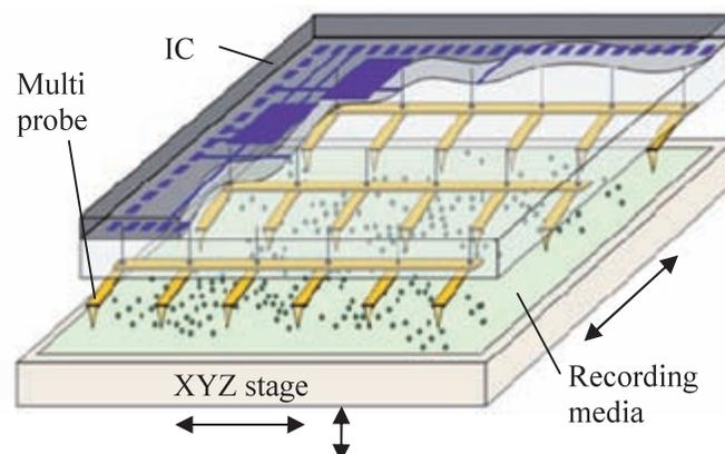
Fig. 2.1. Scanning multiprobe data storage system.
