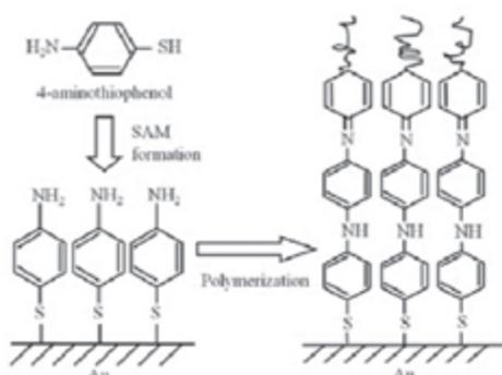
Fig. 2.2. Scheme of surface-graft polymerization of PANI film.
