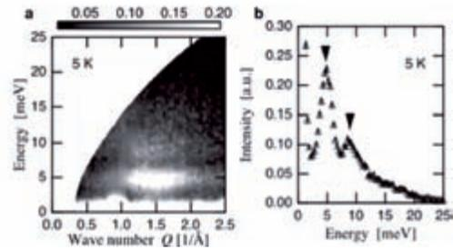
Fig. 4. Resonance-like magnetic peak measured by inelastic scattering on a powder specimen of  $\text{MgCr}_2\text{O}_4$ , (a) contour images in wave number and energy space and (b) energy spectrum at around  $Q=1.5 \text{ \AA}^{-1}$ .
