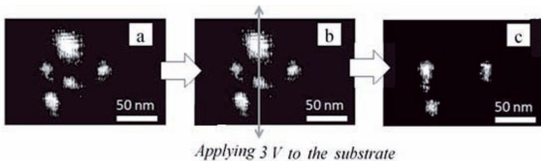
Fig. 2.8. Conductance images of the PANI dots in electrical modification experiment. (a) Before the modification (b) Applying a voltage of 3 V along arrow (c) After the modification
