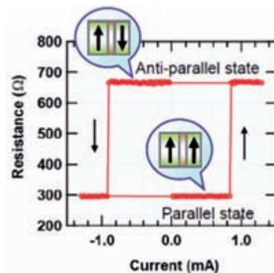
Fig. 6. Typical TMR loop driven by pulsed current.
