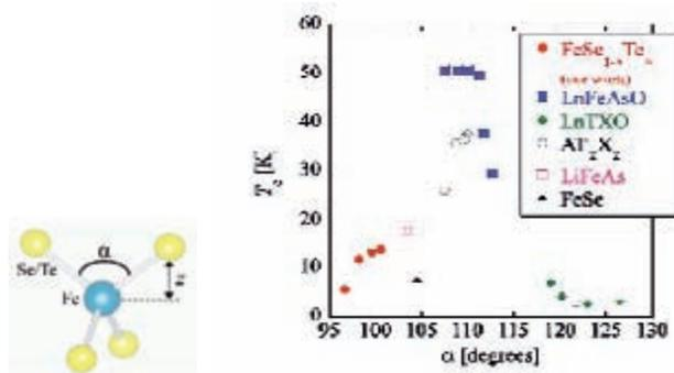
Fig. 7. X-Fe-X (X:As, P, Se and Te) angle  $\alpha$  (left) dependence of superconducting transition temperature  $T_c$ .
