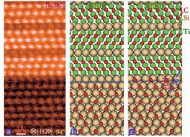
Fig. 2. (a) HAADF-STEM image of the SiC/Ti<sub>3</sub>SiC<sub>2</sub> interface in the ohmic contact sample. The optimized SiC(0001)/Ti<sub>3</sub>SiC<sub>2</sub>(0001) interface models (b) without interfacial C atoms (*SiSi*), and (c) with interfacial C atoms (*SiCSi*) [6].
