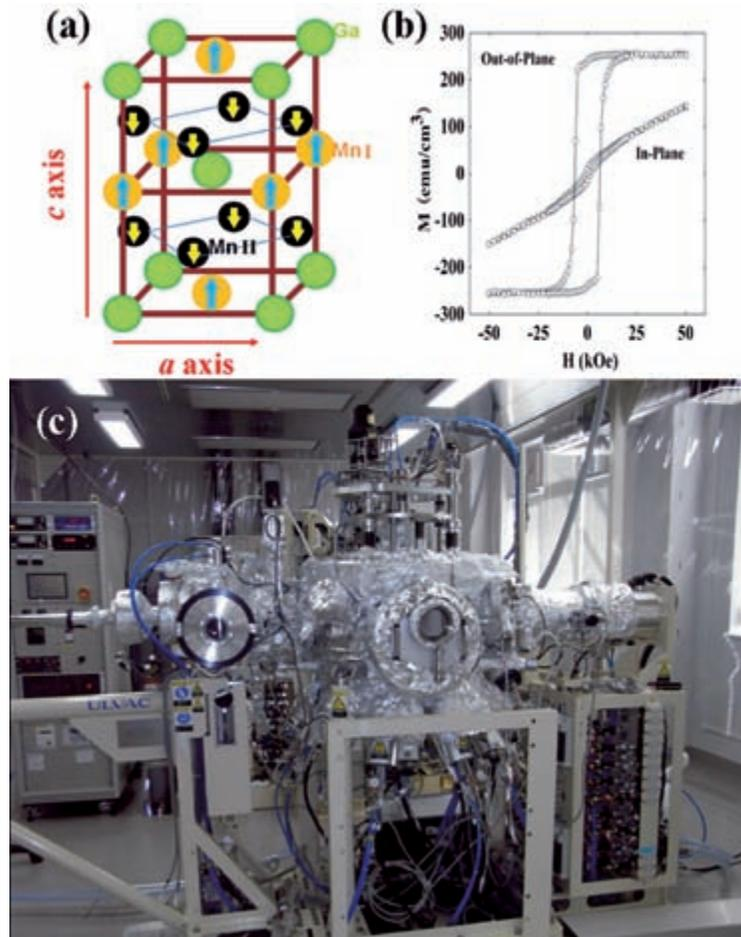
Fig. 4. (a) Crystal and magnetic structure of Mn<sub>3</sub>Ga, (b) Photograph of dc magnetron sputtering equipment, (c)  $M$ - $H$  curves of epitaxial Mn<sub>2.5</sub>Ga films.
