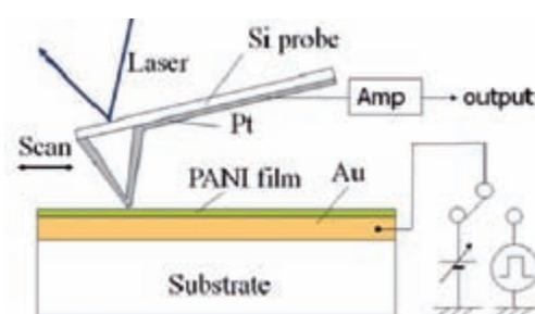
Fig. 2.3. Schematic diagram of the electrical modification experiment with SPM.
