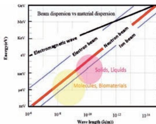
Fig. 3. Matching between beam dispersion and material dispersion for various types of quantum beams
