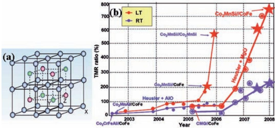
Fig. 3. (a) Crystal structure of Heusler alloy, (b) Development of TMR ratio of the MTJs with Heusler electrodes.
