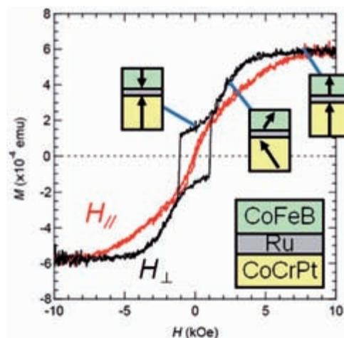
Fig. 8. Magnetization curves of SyF structure with magnetic field in-plane and perpendicular.
