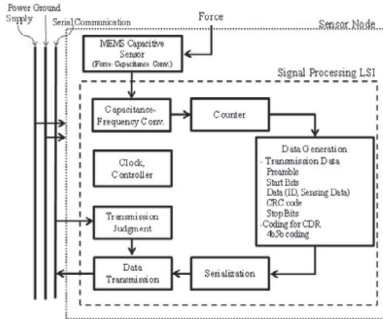
Fig. 3.2. An overview of a sensor node.
