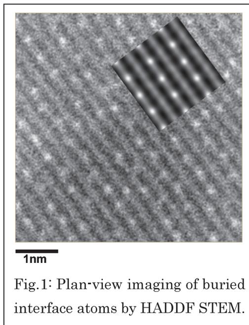
Fig.1: Plan-view imaging of buried interface atoms by HADDF STEM.
