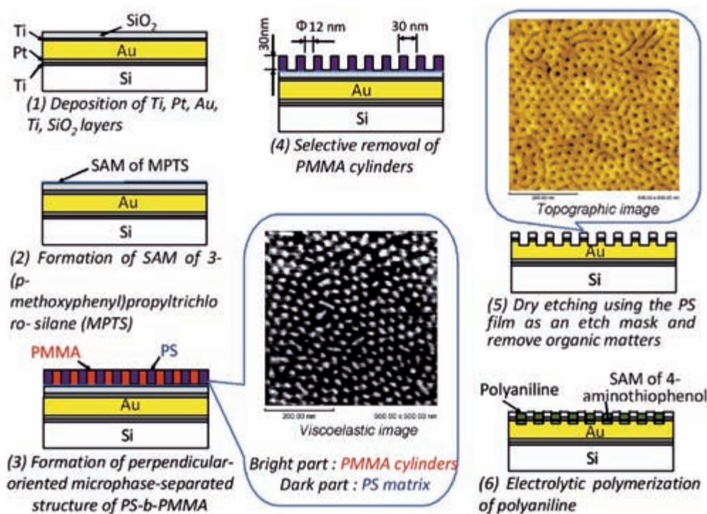
Fig.2.6. Fabrication process of the conductive polymer patterned medium.
