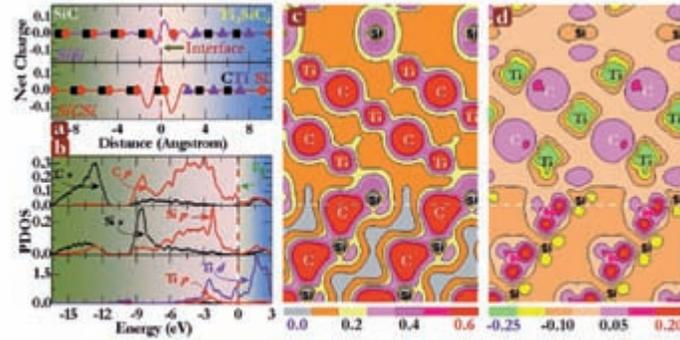
Fig. 3. (a) Planar-averaged charge density along the [0001] direction for the *SiSi* and *SiCSi* interfaces, (b) density of states projected on the atomic layers proximal to the *SiCSi* interface, (c) charge density and (d) its difference along the (1120) plane of the *SiCSi* interface [6].
