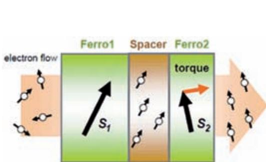
Fig. 5. Schematic illustration of spin transfer torque.
