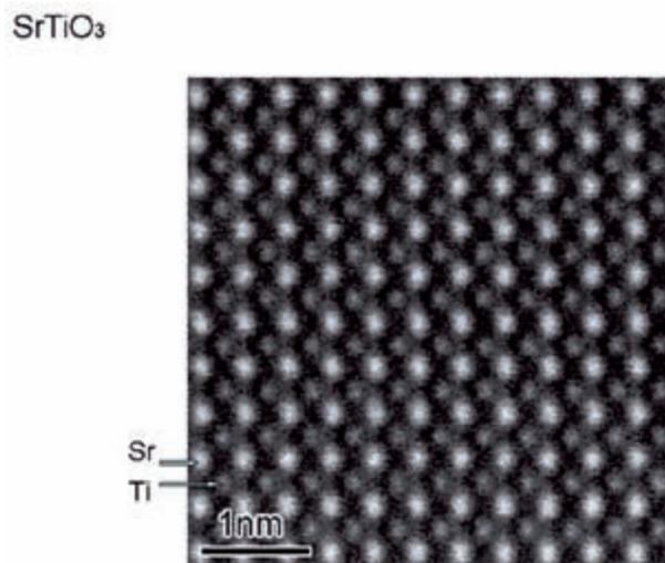
Fig. 1. HAADF-STEM image for  $\text{SrTiO}_3$  projected along the  $[001]$  direction, in which the contrast of Sr atoms ( $Z=38$ ) is brighter than that of Ti atoms ( $Z=22$ ).
