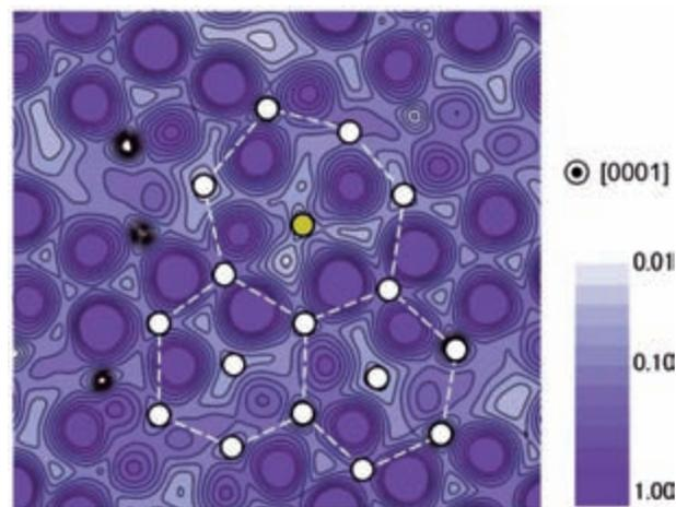
Fig. 8. Electron density map around Y atoms segregated in  $\Sigma 31$   $\text{Al}_2\text{O}_3$  grain boundary, which was obtained by the first principles calculation [14].
