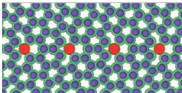
Fig. 6. The stable atomic structure of Pr-doped ZnO  $\Sigma 7$  grain boundary obtained by the first principles calculation (green circle: O, blue circle: Zn, red circle: Pr) [13].
