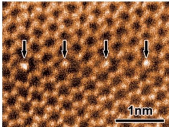
Fig. 5. HAADF-STEM image of Pr-doped ZnO  $\Sigma 7$  grain boundary, showing that Pr segregation sites can be observed as bright spots indicated by the arrows [12].
