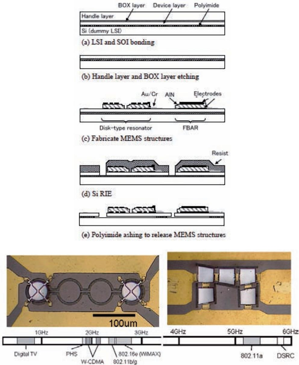
Fig. 1.2. Multi-band AlN filters fabricated on a common chip.
