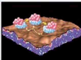
Fig. 1: Schematic diagram of the activation of an STZ in a glassy material. Mechanical failure through macroscopic shear occurs by the accumulation of a critical number of activated STZs on a slip plane.
