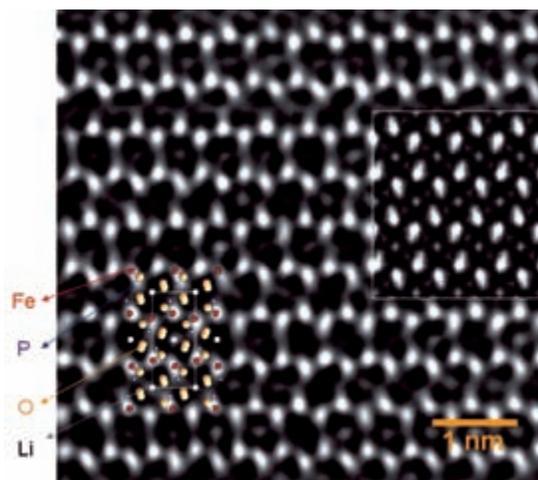
Fig. 13. HAADF-STEM image for the  $\text{LiFePO}_4$  crystals, in which a part of Li sites was exchanged by Fe atoms, showing that some of the Li columns have a bright contrast in significant intensity [20]. The inset shows the simulated HAADF image for the olivine with 15% Li-Fe exchange.
