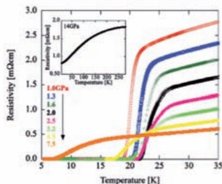
Fig. 8. Superconducting transition in FeSe<sub>0.5</sub>Te<sub>0.5</sub> under high pressure. Inset shows the temperature dependence of electrical resistivity under 14GPa
