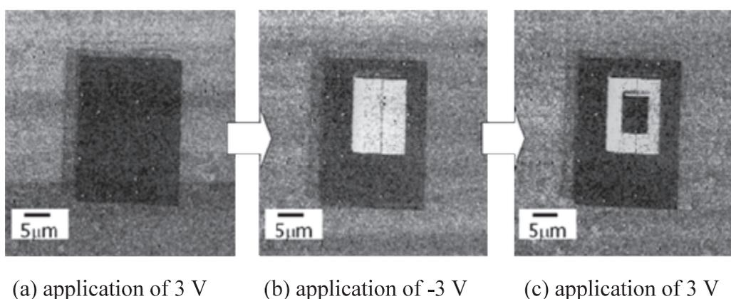
Fig. 2.4. Reversible conductive change of PANI by modification voltage.
