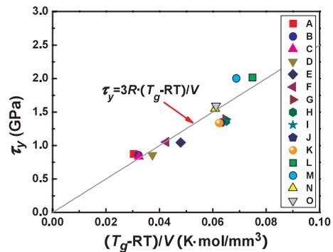
**Figure 1** The relationship between yield shear stress  $\tau_y$  and glass transition temperature  $T_g$ . The solid line is the plot of the linear equation,  $\tau_y=3R\cdot(T_g-RT)/V$ , in which  $R$  is the gas constant. The symbols represent various BMGs used in this study.<sup>5</sup>
