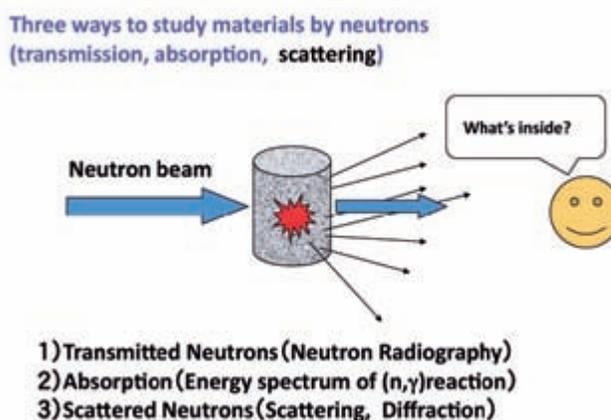
Fig. 1. Typical three techniques to investigate materials by using neutron beam
