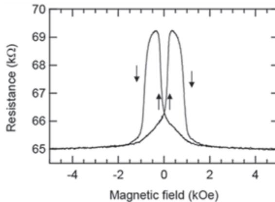
Fig. 9. TMR curves of the MTJ having SyF structures with magnetic field perpendicular.
