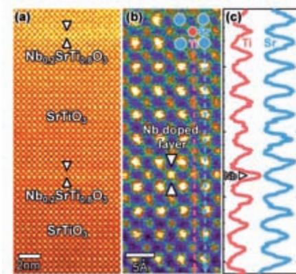
Fig. 11. (a) HAADF-STEM image of SrTiO<sub>3</sub>/Nb-SrTiO<sub>3</sub> superlattice, (b) magnified image of the region (a) and (c) image intensity profile of Ti and Sr layers [19].
