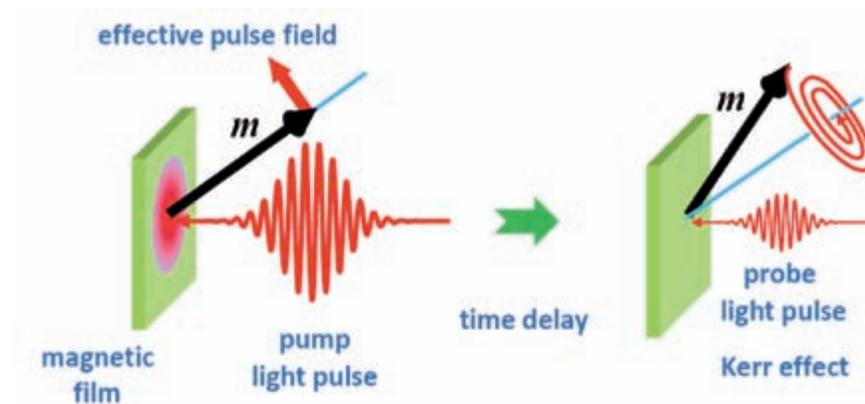
Fig. 10. Schematic illustration of measurement principle of all-optical detection of magnetization precession.
