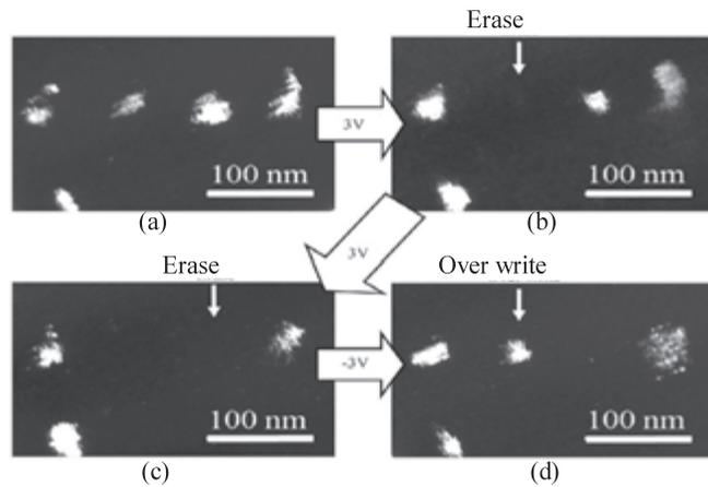
Fig. 2.7. Conductive polymer patterned medium for scanning multiprobe data storage
