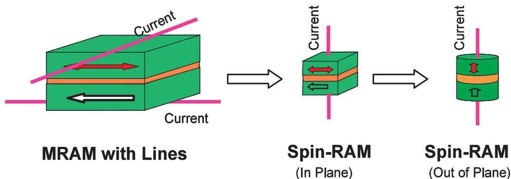
Fig. 2. Change of TMR cell in research of magnetic memory.
