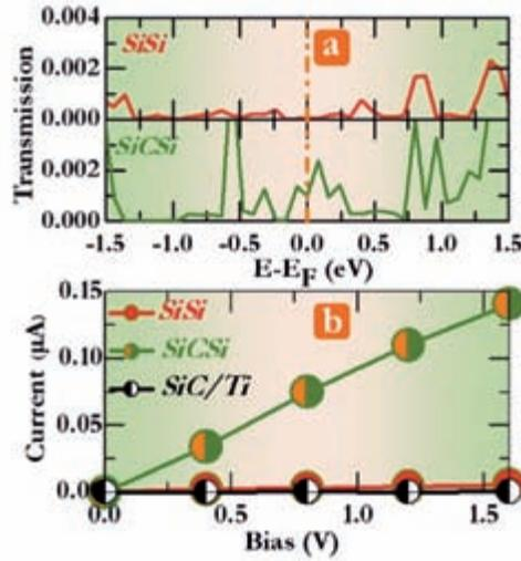
Fig. 4. (a) Transmission spectra under 0 V and (b) current-voltage curves for the two relaxed systems including the *SiSi* and *SiCSi* interfaces [6].
