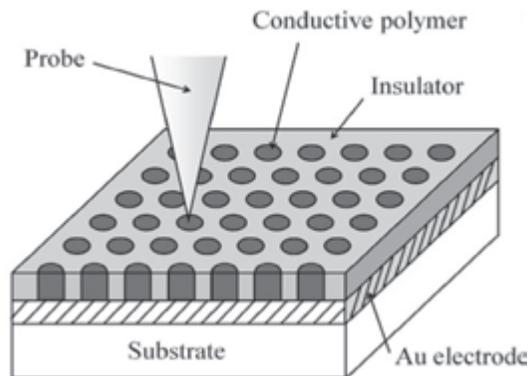
Fig. 2.5. Structure of a conductive polymer patterned medium for scanning multiprobe data storage
