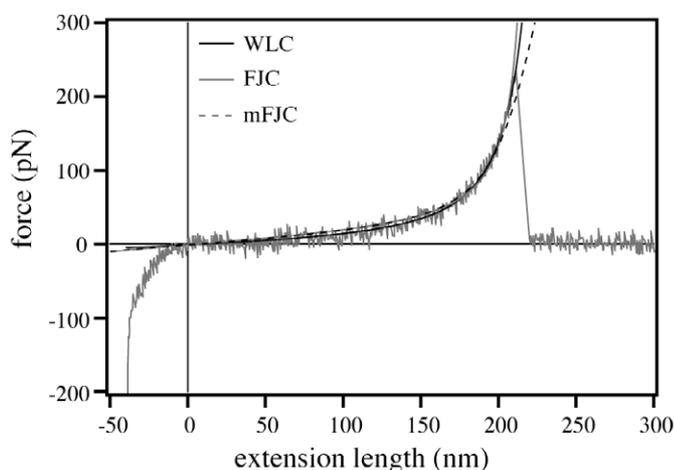
**Figure 8.** Static nanofishing of a single PS chain in cyclohexane. The solvent temperature was about 35°C. WLC (solid black line), FJC (solid grey line) and mFJC (dashed line) models were used to obtain fitting curves.
