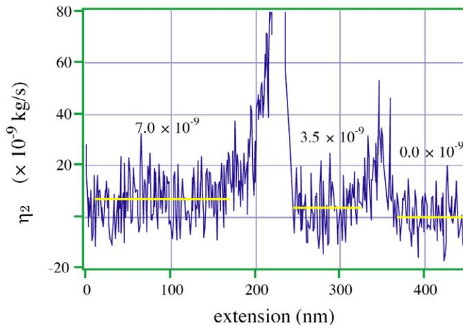
**Figure 10.** Quantized frictional coefficient during stretching two polymer chains at the same time.
