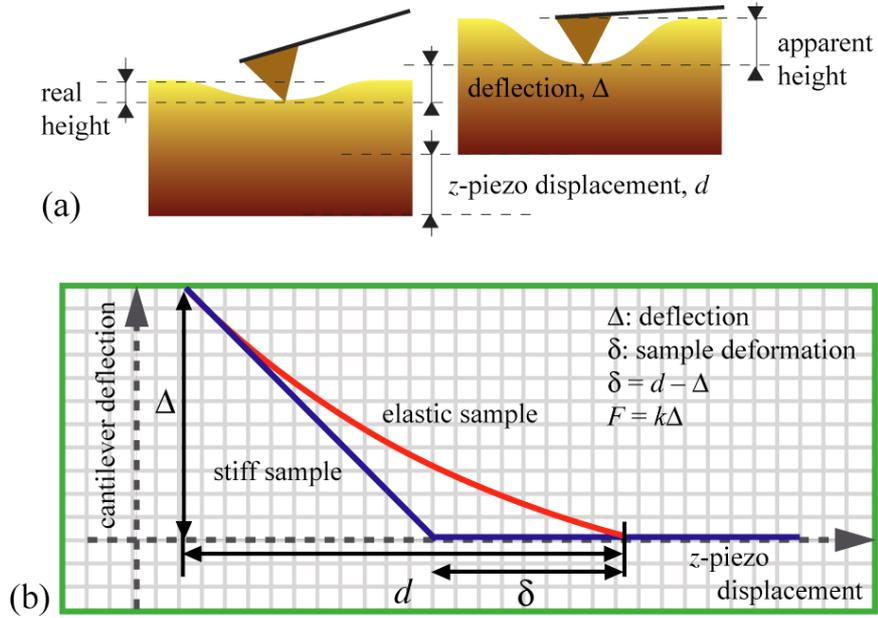
**Figure 4** (a) The schematic drawing of sample deformation for an elastic sample. (b) The comparison between force-distance curves for stiff and elastic samples.
