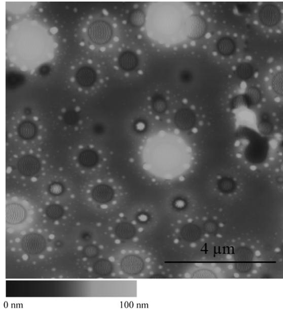
**Figure 5** The height image of a PS/PIB blend thin film on a glass substrate in tapping mode.
