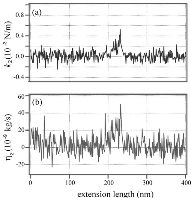
**Figure 9.** The behavior of (a) chain stiffness,  $k_2$  and (b) viscosity of the chain,  $\eta_2$  against the extension. The values were calculated by a double Voigt model.
