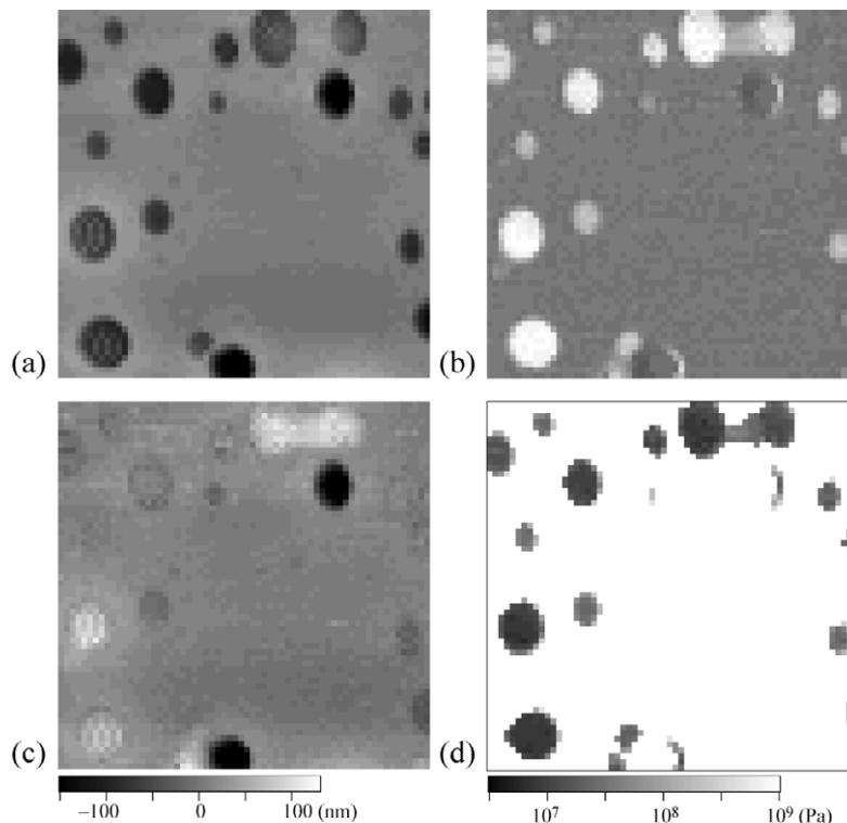
**Figure 6** The result of a force volume measurement on the same sample. (a) The force volume (apparent) height image, (b) the sample deformation image, (c) the reconstructed real height image and (d) the Young's modulus distribution image.<sup>5)</sup>
