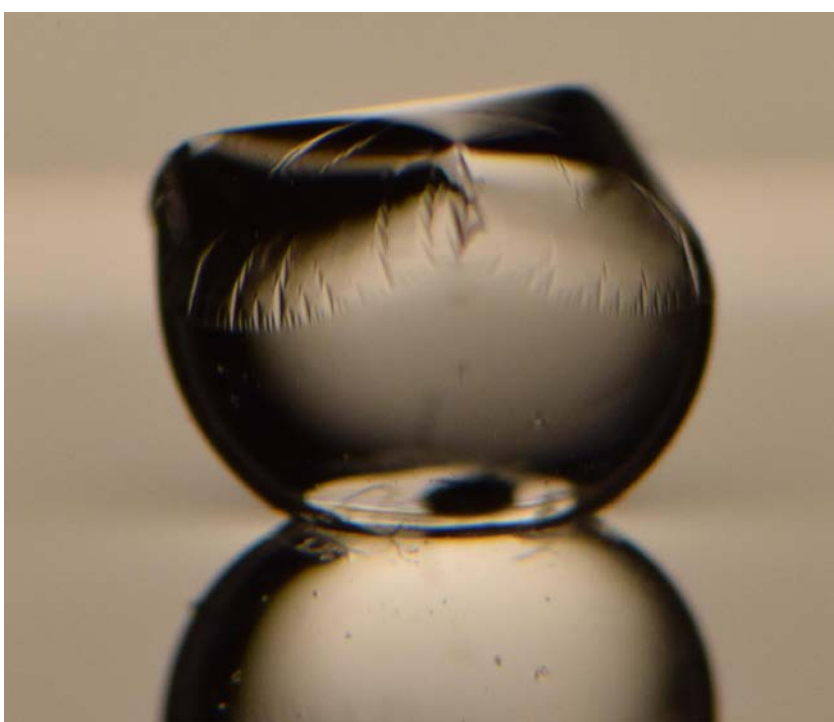
A circular polystyrene sheet, only 39 nanometers thick, partially encloses a water droplet by wrinkling and folding. When placed on a smaller droplet, the sheet forms a shape resembling a stuffed dumpling.
