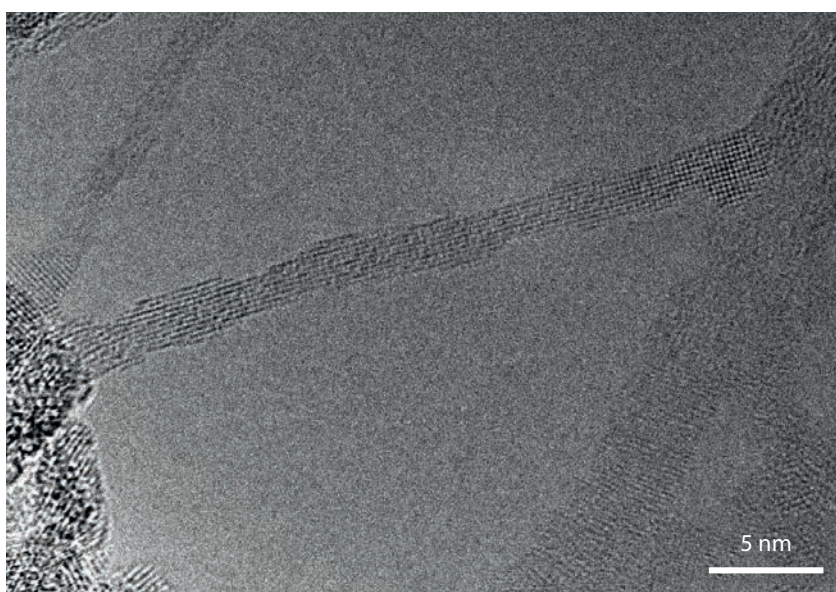
A transmission electron micrograph showing several ultrafine sodium titanate nanowires.
