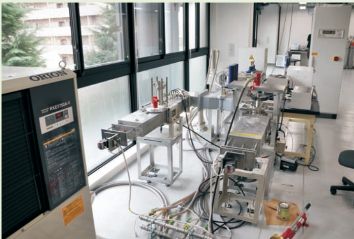
A Single-Mode Applicator for Microwave Processing of Materials under Pressure in a Controlled Atmosphere
