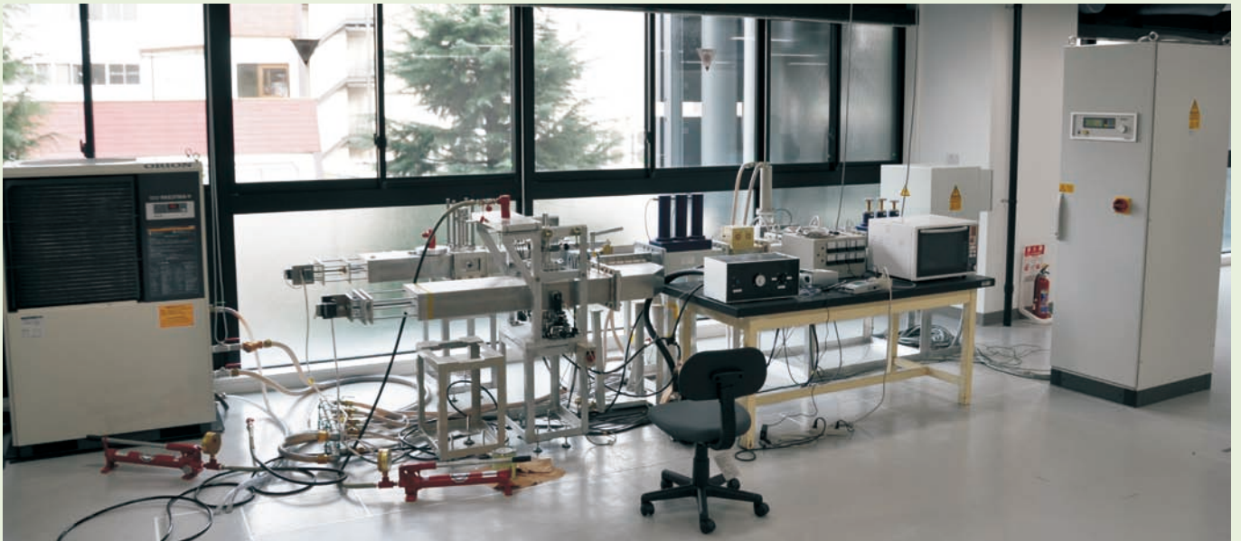
A Single-Mode Applicator for Microwave Processing of Materials under Pressure in a Controlled Atmosphere
